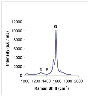
Spectrum obtained with 633 nm laser.
