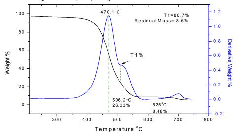
The small peak in the derivative curve above  $625\,^{\circ}\text{C}$  is due to changes in the residual catalyst as the material is heated.
