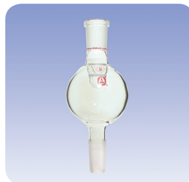
Anticlimb splash-guard adapter with fritted disc
