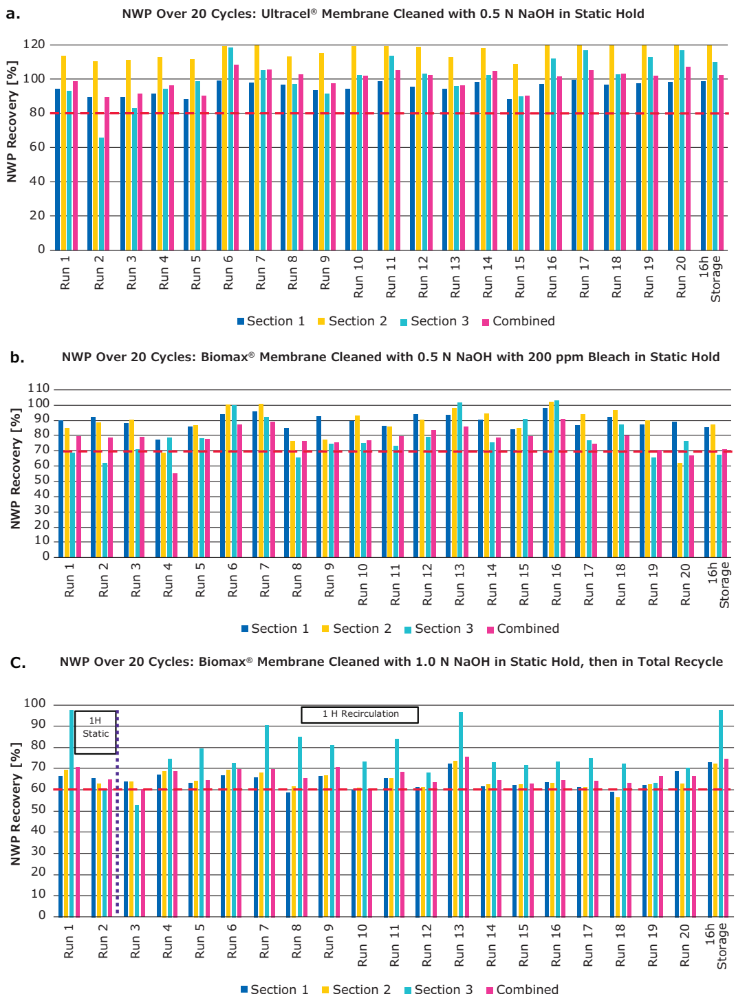
Figure 3. NWP versus process run number for: a) Ultracel® membrane cleaned with NaOH, b) Biomax® membrane cleaned with NaOH and bleach, c) Biomax® membrane cleaned with NaOH.
