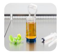
Install the needle guide onto the top of the canister.
