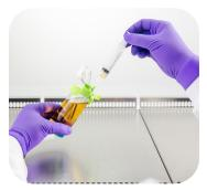
Attach the provided needle to a syringe and guide the needle into and through the canister's chimney, thereby piercing the tubing of the canister.
