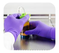
After sampling, close the clamp of the needle guide to keep your canister safe from external contaminants.
