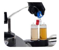
At the end of the sterility test workflow, close the clamps and cut the tubing.
