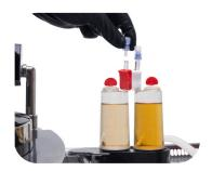
Install the needle-free valve onto the cut tubing of each canister and place the red plug onto the vent.
