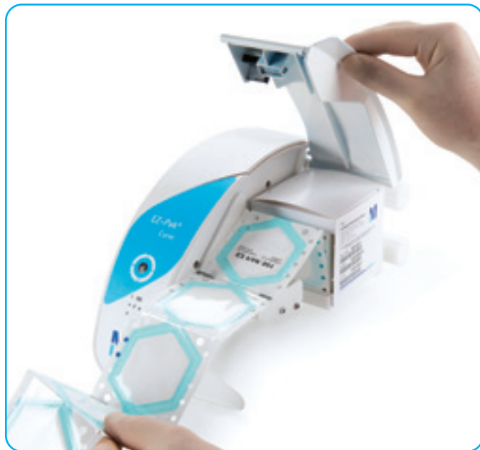
Step 2 Pull the roll out until the first membrane is visible, then cover.
