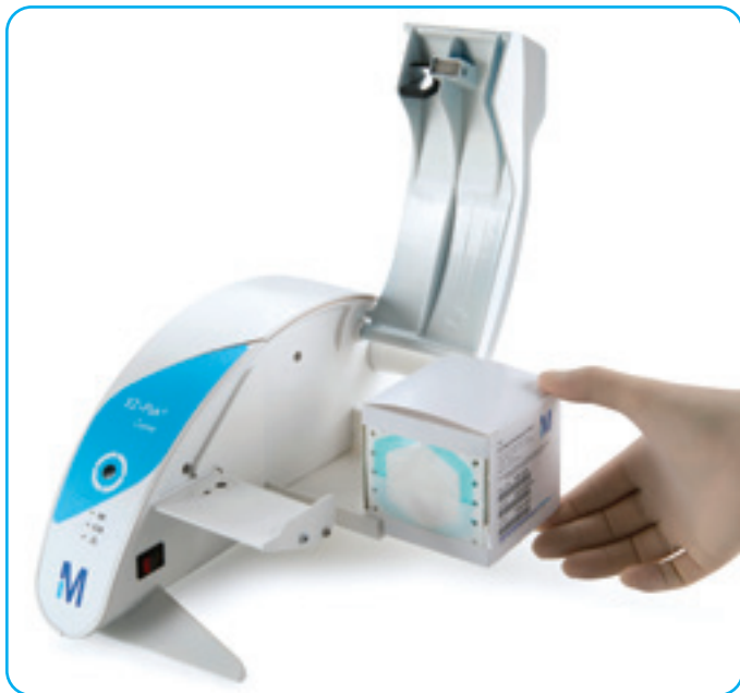
Step 1 Open cover and insert the cartridge.
