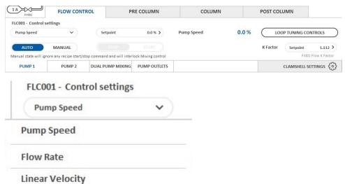
The flow can be controlled by a fixed speed value for the pump:
