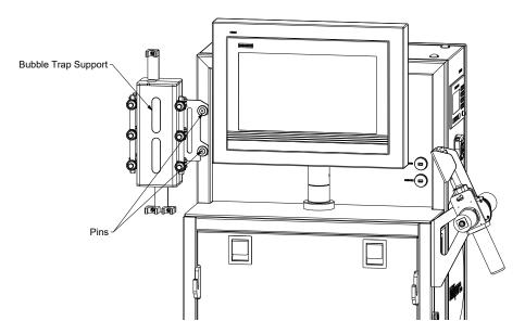
Installing the BBT Support on the Base
