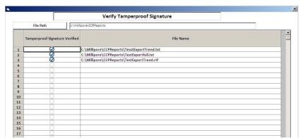
The files with the check marks are the original files created by CCP® software using the unalterable raw data archived during the run. The unchecked report files were altered in some way by software outside the CCP® system.
