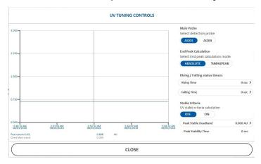
Note Peak detection is used to automatically identify when the product is coming outside of a column in order to isolate it in specific containers (fraction outlet).
