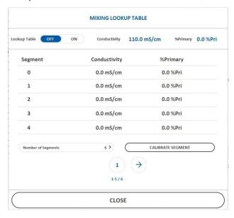
The Mixing Lookup Table allows to minimize the conductivity control error when performing conductivity gradient (step or linear). The table compensates for the nonlinear relationship between mixing percentage and measured conductivity.
