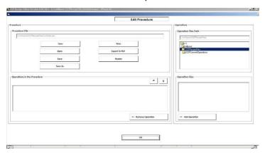
In the lower right corner of the form, the Operation Files list box presents all the operations currently stored within the path indicated in the Operation Files Path list box. To add an Operation to the Procedure, select the Operation from the list of Operations on the right and click the Add Operation Button. The Operation is added to the Operations in the Procedure list box located in the lower left corner of the form. To remove operations from this list, click on Remove Operation.
