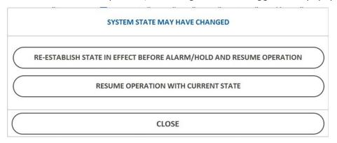
The first option « Re-establish state in effect before alarm/hold and resume operation » allows to restore the flowpath, pump status, in place before the alarm so that the process can restart at its previous state.
