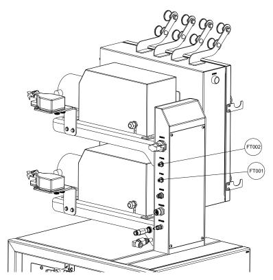
Flowmeter Transmitter Connections
