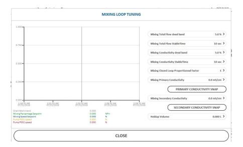
The Mixing Loop Tuning popup shows the control loop values. Tune the control parameters to reach the desired dynamic properties.
