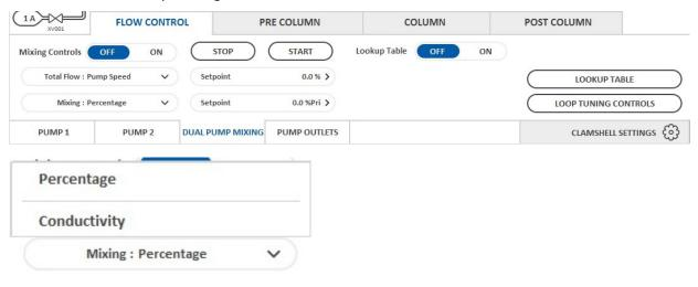
One of the capabilities of the system is the ability to form gradients based on conductivity. It allows a gradient to be defined in terms of the conductivity (in  $\mu$ S) of the fluid entering the column. The software employs a hybrid feed-forward-feedback algorithm to manipulate the gradient valve to achieve the desired conductivity.
