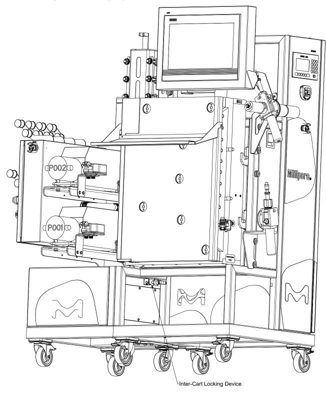
Connecting the Pump Cart with the Base
