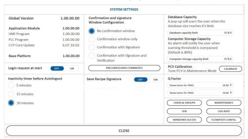
Click the CALIBRATE button to start the calibration (the label of the button changes to "In progress" and wait until the button returns to its initial label.
