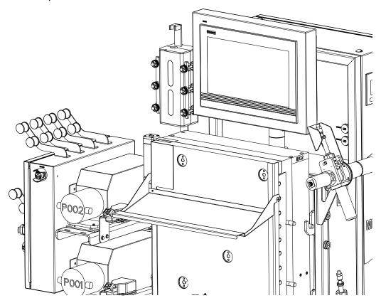
Installing the Keyboard Holder
