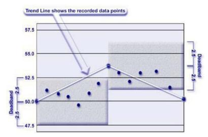
The first recorded value shown is 50. The next value that Historical Collect records must be greater than or equal to 52.5 or less than or equal to 47.5.
