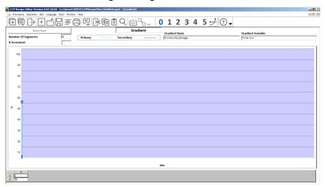
Clicking on the Gradient Basis entry box allows one to base the formation of the gradient on primary percentage or conductivity.
