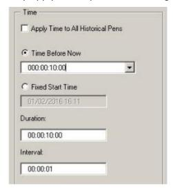
Time Before Now has a drop-down menu that allows the user to choose the time period from current time. There are five choices: One hour, Two hours, Four hours, Eight hours and Twenty-Four hours.
