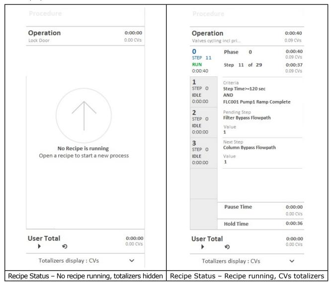
When a recipe is running, the left part of the display shows the following information for each phase tab:
