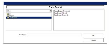
To open a report, select the file from the list on the right side of the form and click OK. The File Name can be typed in the text box provided on the bottom of the form. The selected report is opened within the corresponding application.
