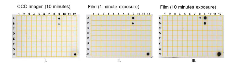
Figure 3: Comparison of detection with CCD imager and film
