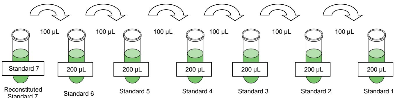
After serial dilutions, the tubes should have the following concentrations for constructing standard curves.
