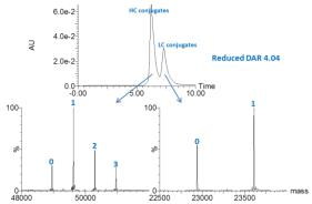
50 mM DTT for 1 hour at 37 °C 2 mm  $\times$  30 cm TSKgel SuperSW3000 SEC column isocratic 70  $\mu$ L/min, 30% ACN with 0.1% TFA 2  $\mu$ g injection Xevo G2 QToF 400–4000 m/z
