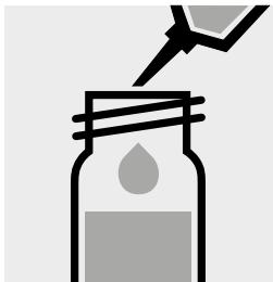
Add 6.0 ml of **B-6** with pipette, close with the screw cap, and mix.
