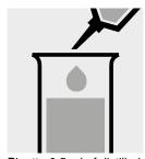
Pipette 0.5 ml of distilled water (Water for analysis EMSURE®, Cat.No. 1.16754, is recommended) into a plastic vessel.
