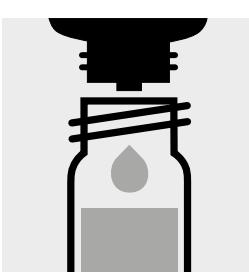
Add 5 drops of Ag-5, close with the screw cap, and mix.
