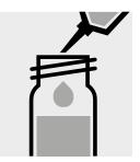
Add 5.0 ml of the close the cell with the screw cap, and mix.
