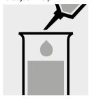
Add to each tube 0.20 ml Transfer both solutions of CI-2 with pipette and mix.
