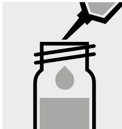
Add 1.0 ml of the sample with pipette, close the cell with the screw cap, and mix.
