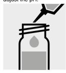
Add 2.5 ml of **SO<sub>4</sub>-3** with pipette and mix.
