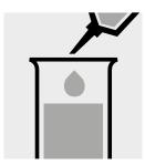
Add 0.20 ml perchloric acid 70 - 72 % GR (Cat.No. 1.00519) with pipette and mix.
