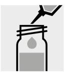
Pipette 0.20 ml of AOX-1K into a reaction cell, and mix.
