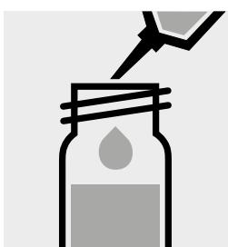
Add 1.0 ml of **OA-4K** with pipette, close the cell with the screw cap, and shake vigorously.
