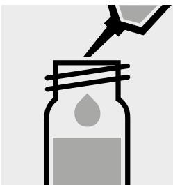
Add 1.0 ml of H-1K with pipette, close the cell with the screw cap, and mix.
