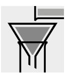
Filter the entire mixture over a hydrophobic filter acc. to ÉN 1141 [1] or §64 LFGB 31.00-7 [2]: reagent blank.
