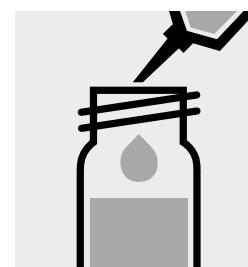
Add 2.0 ml of **hydrochloric acid 6 mol/l** with pipette, close the vessel, and mix.
