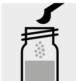
Add 1 level grey micro-spoon of **TOC-2K**. **Immediately** close the cell tightly with an **aluminium cap** (Cat.No. 1.73500).
