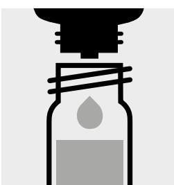
Add 2 drops of **Cl<sub>2</sub>-3**, close with the screw cap, and mix.
