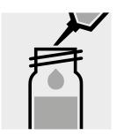
Add 8.0 ml of sodium hydroxide solution 2.5 mol/l with pipette and mix.
