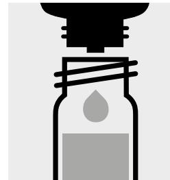
Add 6 drops of **K-1K**, close the cell with the screw cap, and mix.
