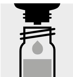
Add 2 drops of **reagent 2**, close the cell with the screw cap, and mix.
