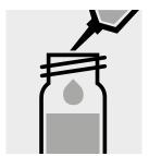
Add 10 ml of n-butyl acetate and close the test tube with the screw сар.
