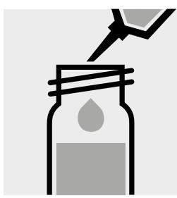
Add 0.80 ml of **B-3** with pipette, close with the screw cap, and mix.
