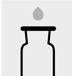
Fill 2 oxygen reaction bottles each with **pretreated sample** and 2 glass beads to overflowing. Close bubble-free with the slanted ground-glass stoppers.
