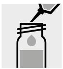
Add 0.25 ml of **Al-2K** with pipette, close with the screw cap, and mix.
