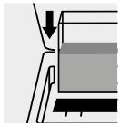
Insert the blank cell into the cell compartment.
