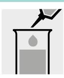
Add 0.20 ml of reagent 2 with pipette and mix.
