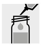
Add 5.0 ml toluene GR (Cat.No. 1.08325) with pipette, close the cell with the screw cap.
