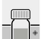
Cool the vessel in an ice bath/water bath for **exactly** 10 minutes.
