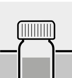
Temper the vessel in a water bath at  $95 \pm 5$  °C for **exactly** 10 minutes.
