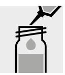
Add 2.0 ml of ninhydrin solution, close the test tube with the screw cap, and mix.
