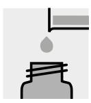
Add approx. 30 ml of boiling ethanol (w = 90 %) and allow to cool to room temperature.
