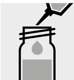
Add 1.0 ml of **OA-4** with pipette, close the cell with the screw cap, and mix.
