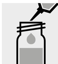
Add 2.0 ml of **ethylene glycol monomethyl ether**, close the test tube with the screw cap, and mix.
