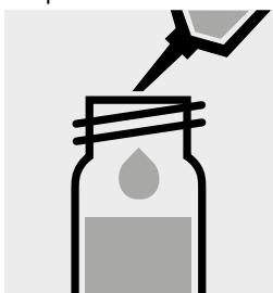
Add 7.0 ml of distilled water with pipette to the second reaction cell, close with the screw cap, and mix.
