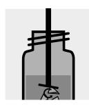
Disintegrate the filter in the homogenizer.
