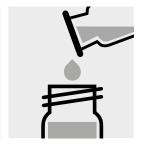
Fill the solution into a round cell.
