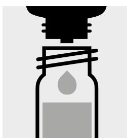
Add 3 drops of Ag-3, close with the screw cap, and mix.
