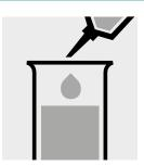
Pipette 10 ml of the pretreated sample into a test tube.
