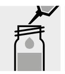
Add 0.20 ml of **Cd-1K** with pipette, close the cell with the screw cap, and mix.
