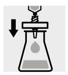
Filter or centrifuge turbid samples.
