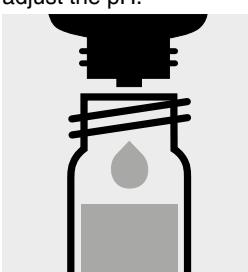
Add 5 drops of **Zn-3K**, close the cell with the screw cap, and mix.
