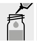
Pipette 0.50 ml of **OA-1K** Add 0.50 ml of the sample with pipette, close with the screw cap, and mix.
