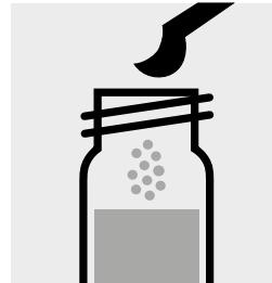
Add 1 level green micro-spoon of  $\text{SO}_4\text{-1K}$ , close the cell with the screw cap.
