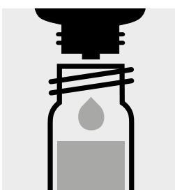
Add 1 drop of Ag-4, close with the screw cap, and mix.
