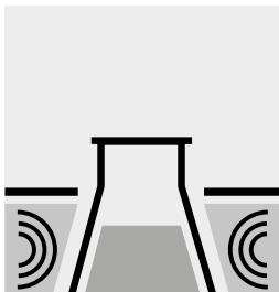
Contains the sample air or gas bubbles: degassing in ultrasonic bath.
