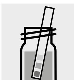
Check the pH, specified range: pH 4 – 10. If required, add dilute sodium hydroxide solution or sulfuric acid drop by drop to adjust the pH.
