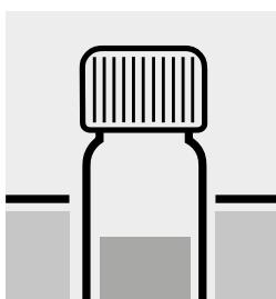
Incubate the test tube in a water bath acc. to EN 1141 [1] or §64 LFGB 31.00-7 [2].
