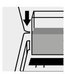
Insert the cell containing the sample into the cell compartment.
