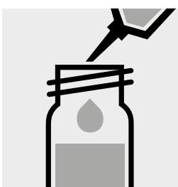
Add 5.0 ml **toluene GR** (Cat.No. 1.08325) with pipette, close the cell with the screw cap.
