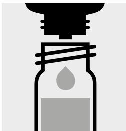
Add 2 drops of **reagent 1**, close the cell with the screw cap, and mix.
