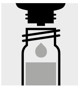
Add 3 drops of **Zn-4**, close the test tube with the screw cap, and mix.
