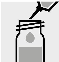
Add 1.0 ml **phosphoric acid 85 % GR** (Cat.No. 1.00573) with pipette, close the cell with the screw cap, and mix.
