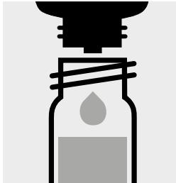
Add 5 drops of **Zn-1K** into a reaction cell, close with the screw cap, and mix.
