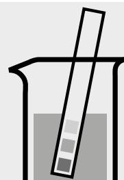
Check the pH of the sample, specified range: pH 3 – 9.
