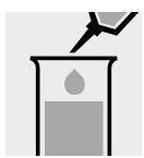
Pipette 4.0 ml of the sample into a test tube.
