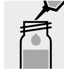
Add 8.0 ml of **sodium hydroxide solution 2.5 mol/l** with pipette and mix.
