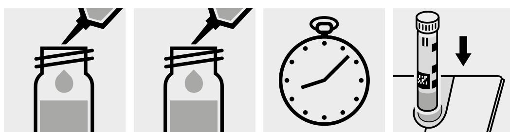
Pipette 0.20 ml of **AOX-1K** into a reaction cell, and mix.
