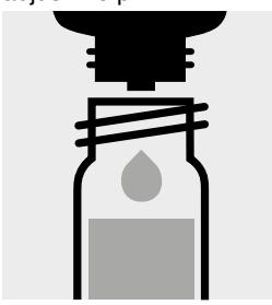
Add 5 drops of **Zn-3**, close the test tube with the screw cap, and mix.
