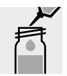
Pipette 2.0 ml of the sample into a reaction cell, close with the screw cap, and mix.
