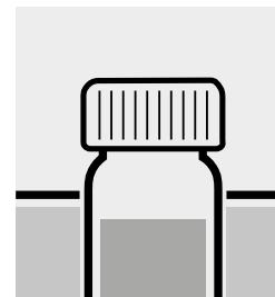
Temper the vessel in a water bath at  $95 \pm 5$  °C for **exactly** 5 minutes.
