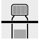
Remove the cell from the thermoreactor and place in a test-tube rack to cool.
