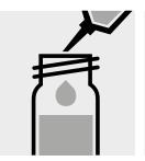
Pipette 5.0 ml of the sample into a reaction cell, close with the screw cap, and mix.
