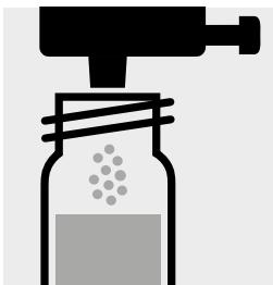
Add 1 dose of NH<sub>4</sub>-1K using the blue dose-metering cap, close the cell with the screw cap.
