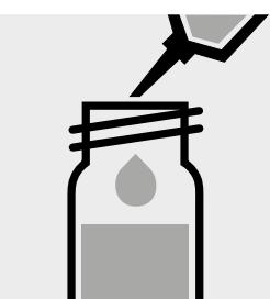
Pipette 1.0 ml of pre-treated sample into a test tube with screw cap.
