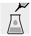
Add 1.0 ml of **As-6** with pipette to the solution in the Erlenmeyer flask and mix.
