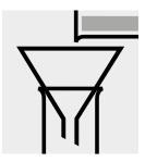
Transfer the residue to a 25-ml volumetric flask using a little distilled water (Water for analysis EMSURE®, Cat.No. 1.16754, is recommended)
