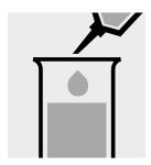
Pipette 0.50 ml of SO<sub>4</sub>-1 into a test tube.
