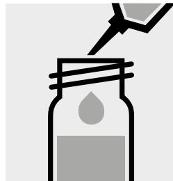
Pipette 0.50 ml of **Zn-2K** into a reaction cell, close with the screw cap, and mix.
