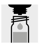
Add 1 drop of Ag-4, close with the screw cap, and mix.
