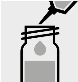
Pipette 4.0 ml of the sample into a reaction cell, close with the screw cap, and mix.
