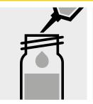
Pipette 2.0 ml of distilled water (Water for analysis EMSURE®, Cat.No. 1.16754, is recommended) into a closable vessel (20 ml).
