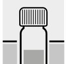
Incubate the test tube in a water bath acc. to EN 1141 [1] or §64 LFGB 31.00-7 [2].
