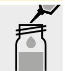
Add 2.0 ml of hydrochloric acid 6 mol/l with pipette, close the vessel, and mix.
