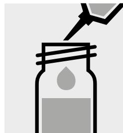
Add 2.0 ml of **DNSA reagent** with pipette, close the vessel, and mix.
