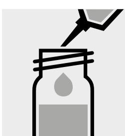
Add 1.0 ml of Ag-6, close with the screw cap, and mix.
