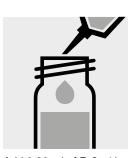
Add 0.80 ml of **B-3** with pipette, close with the screw cap, and mix.
