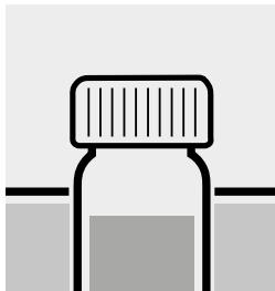
Temper the vessel in a water bath at  $95 \pm 5$  °C for **exactly** 5 minutes.
