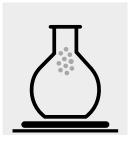
Weigh pulverized sample into a volumetric flask, accurately weighed LFGB 57.22.99-2 [2]. to 0.1 mg.
