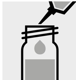
Add 5.0 ml of the sample with pipette, close with the screw cap.
