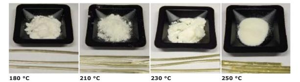
Figure 7: Visual comparison of Parteck<sup>®</sup> MXP extrudate at various temperatures
