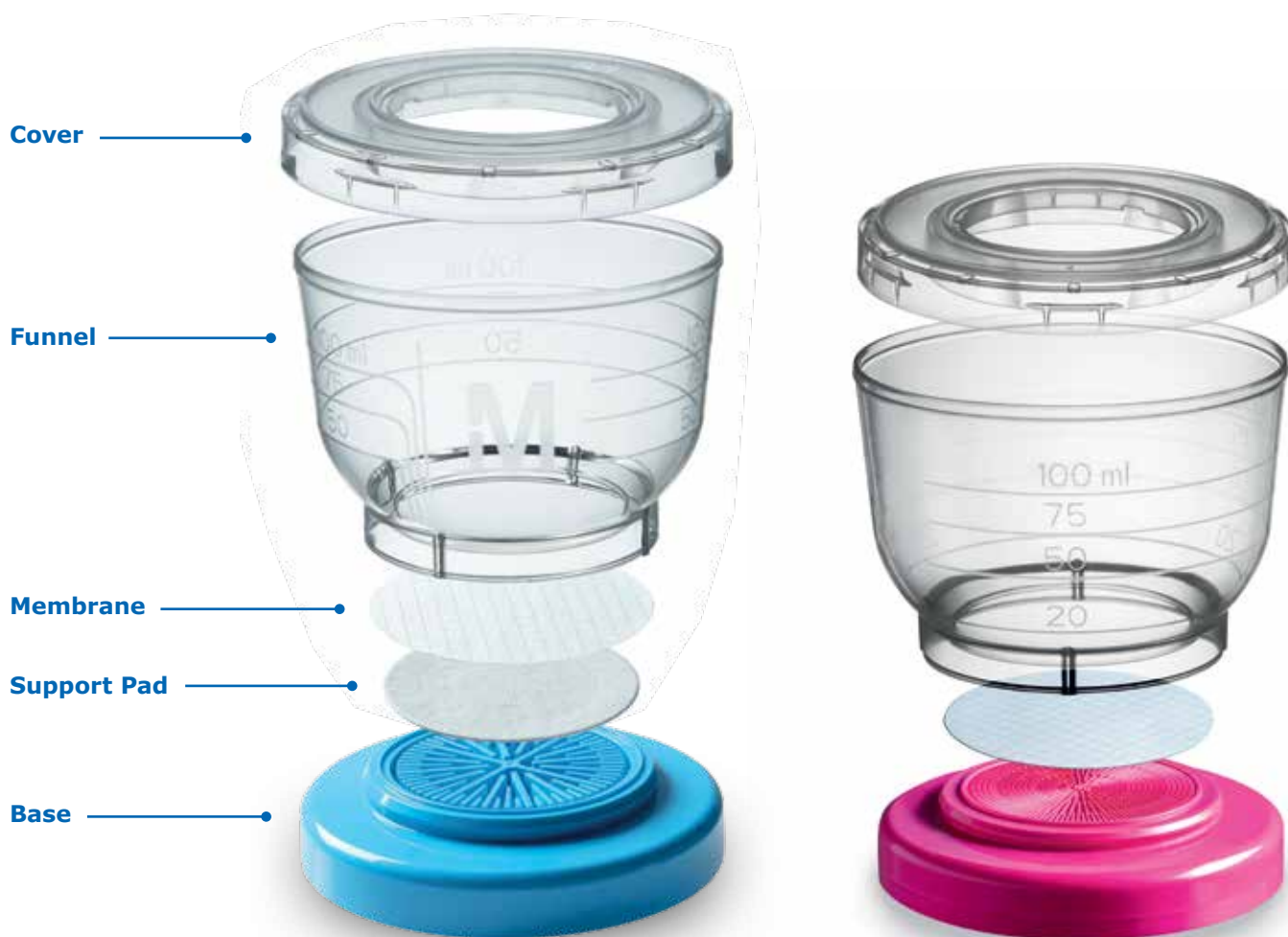
EZ-Fit™ filtration unit components
