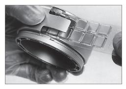
Label the agar strip with the most relevant sample data to avoid problems of identification.
