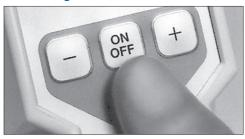
After the required volume has been set, the air sampler is started by pressing the [ON/OFF] key or using the remote control. Starting the instrument with the remote control is possible only after
