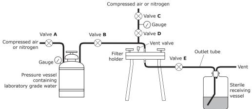
**NOTE:** Filter holder outlet tube or receiving vessel must have a clear portion in order to determine when the bubble point has been reached.
