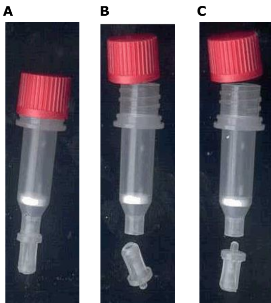
Figure 2. (A) Column, (B) Open column and snapped off tip and (C) Inverted broken tip serves as column closure.
