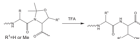
Fig. 1: Conversion of a pseudoproline residue to a Ser or Thr residue.
