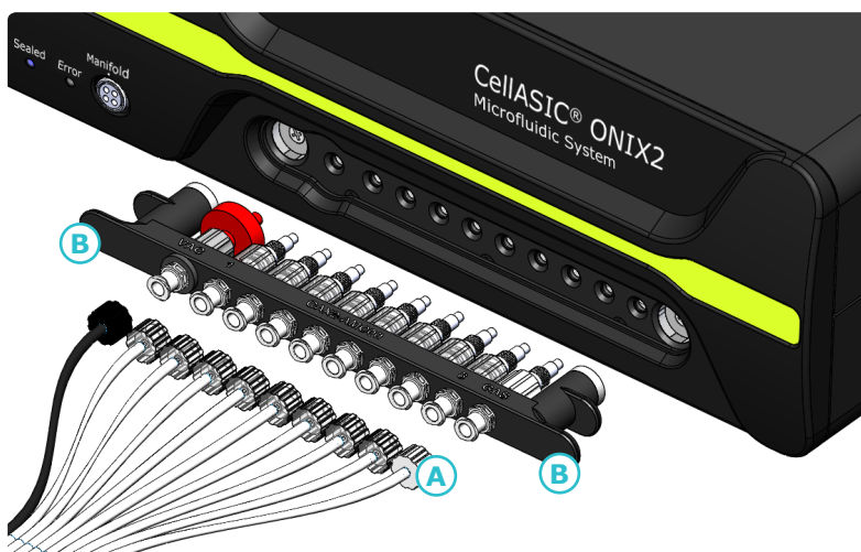
Figure 6. Connecting the Filter Multiconnector
