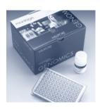
Montage and MultiScreen Sequencing Reaction Cleanup products incorporate patented size-exclusion membrane to yield highly purified sequencing reaction products. In addition to eliminating centrifugation steps, filter plates do not require filtrate collection or column packing.
