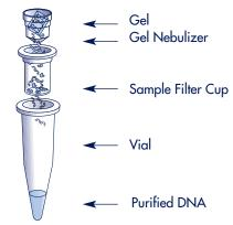
Exploded view of Ultrafree-DA centrifugal unit.
