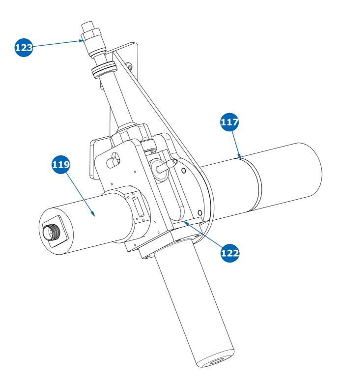
XMO1/2 & XMO3 Single-Use Pre-Column Instrumentation (pH/Conductivity)
