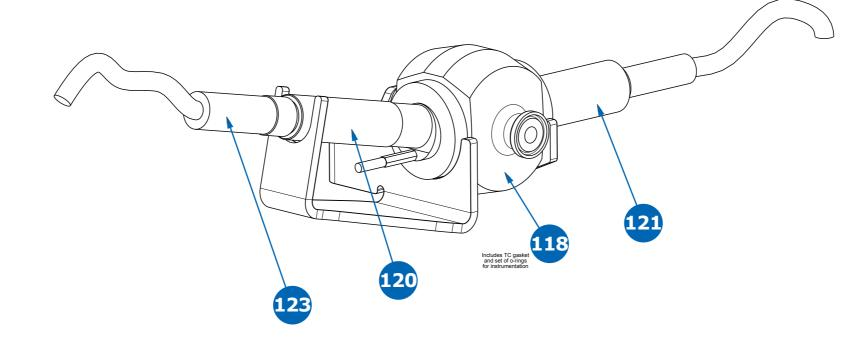
XMO1/2 & XMO3 Single-Use Post-Column Instrumentation (pH/UV/Conductivity)
