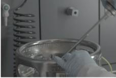
The solvent container must be closed tightly with the original screw cap by using an appropriate key (1.08803.0001).
