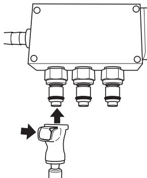
Insert the output tubing onto the stainless steel connector.
