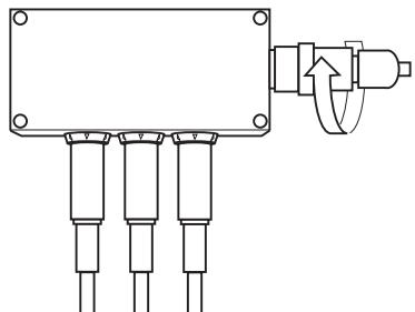
To disconnect the electrical cables from the hub, pull the cables out of the hub.
