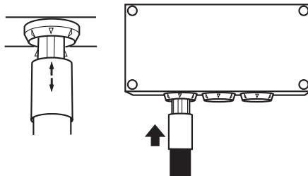
Connect the power supply to the electrical hub and tighten the connector.
