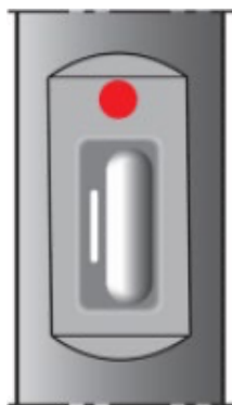
Replace battery* *Once the Red Icon shows up, please change the battery.
