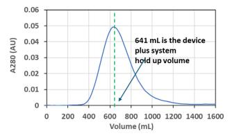
Example of a chromatogram showing  $UV_{280}$  of a 2% acetone pulse used to measure the system hold-up volume
