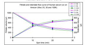
Samples were spun at room temperature, in a swinging bucket rotor at 3000 x g for the times indicated for the 3 different molecular weight cut off devices. Both the Filtrate (F) and retentate (R) volumes are shown.
