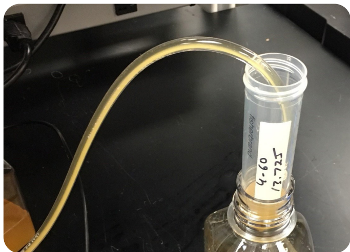
Figure 3. Settling of cell culture in tubing. Feed stream: CHO cell culture harvest (mAb05, 9.7 \times 10^6 TC/mL, 62% viability). A 1/8 in i.d. pump tubing at a flowrate of 2.5 mL and total runtime of 60 minutes is shown (system residence time: 7 minutes).
