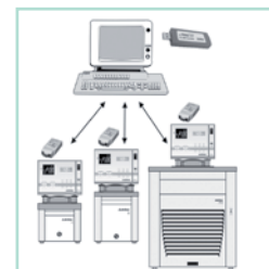
PC and Wireless PC USB Stick to control and monitor up to 8 JULABO instruments
