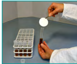
2. Filter inkubieren, optional (BCYE, 36±2°C)
