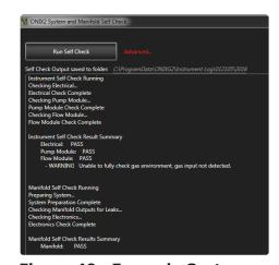
Figure 40. Example System and Manifold self check result with a gas input warning
