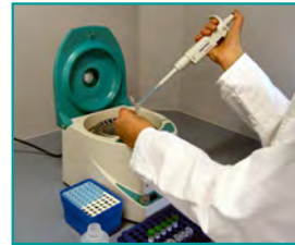
3. Zell-Lyse (2 ml Probe, 13.000 rpm; 37°C, 45 min)
