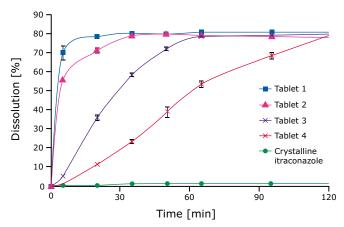
Dissolution method: FDA-recommended conditions for itraconazole, 900 mL SGF, 37 °C, 100 rpm, formulated extrudate with 30% drug load; n=3  $\,$
