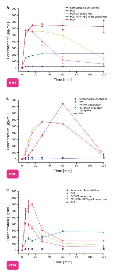
A comparison of the results for the hot melt extruded formulations and the DSC screening methods showed difference in release characteristics (Figure 5). In the study, PVA extrudates generated high supersaturation both in the screening method and the HME; the PVP and polyvinylpyrrolidone-vinyl acetate copolymer (PVP/VA) behaved in a similar manner in both methods, whereas the graft copolymer showed a low performance in both.
