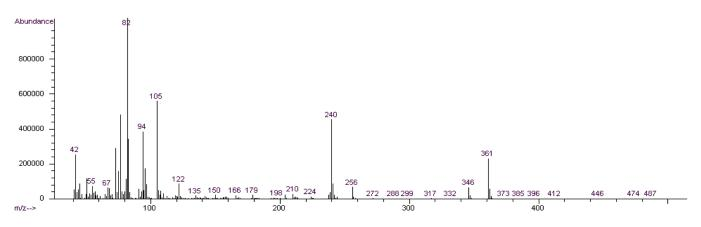
70 eV Electron Ionization Mass Spectrum
