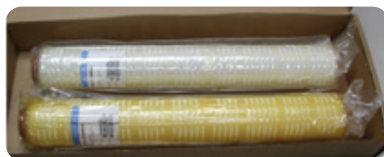
Figure 2. Milligard® cartridge that was kept at recommended storage conditions (top) compared with one that has been exposed to excess heat and/or humidity (bottom).
