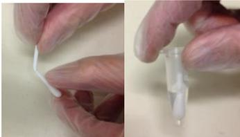
1. A cotton swab is used to wipe a particular surface of the detection area. The swab is then inserted into 0.5mL of distilled water for an immediate test, or into 0.5mL of incubation solution for an incubation period ranging from 3 to 10 hours at 38.5°C, before measuring. Add an enzyme inducer after inserting the swab into the water or incubation solution.
