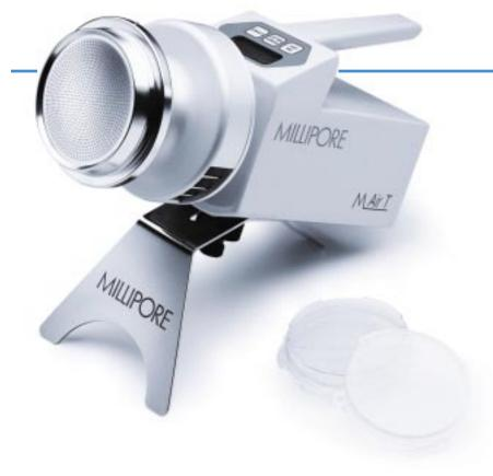
The M Air T is a lightweight, portable system for testing the microbial quality of air in clean rooms, barrier environments, and critical filling areas. The tester is small enough to be used in confined spaces, but powerful enough to sample up to 1000 liters in just 7 minutes. Programmable electronics and unique, ready-to-use agar cassettes make it the most convenient method for active air monitoring.
