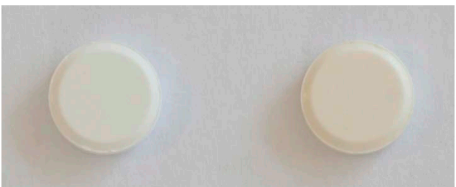
Figure 4: Colour of “Product A” tablets (upper tablet) vs. Pardeck® ODT tablet after 26 weeks storage at 40 °C/75% r.H.
