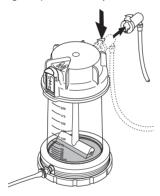
5. Remove stir bar and recover concentrated sample. Save filtrate sample if required.
