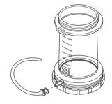
5. Insert stir bar into cell body until support ring is seated on ridge inside the top of cell body.
