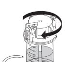
10. Attach pressure inlet tubing assembly by inserting female connector onto quick-connect fitting on cap until it clicks.
