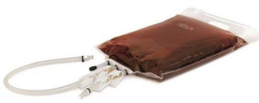
Vegetable Peptone Broth is a universal complex medium for the isolation and cultivation of microorganisms, especially for the microbiological validation of aseptic filling processes (Media Fill Test).
