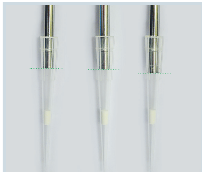
Fig. 5: Insertion depth of a testing prod in 20 µL tips of manufacturer G. All tips were taken from same box.
