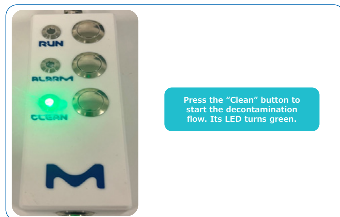
Figure 19: Control box - Clean (decontamination) in progress
