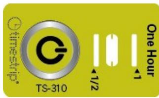
The Timestrip® 1 Hour indicator monitors time elapsed over a period of one hour. It is designed to be used at room temperature conditions. It is inert until activated and can be stored at room temperature until needed. It is self-adhesive, single use and irreversible. It has a pre-activation shelf life of two years from shipping.
