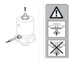
5. Keeping air supply position, installthe actuator to the valvebody.
