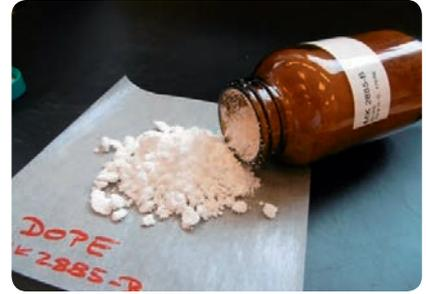
**Figure 4.** Wax-like, amorphous DOPE in comparison to free flowing powder DOPE.
