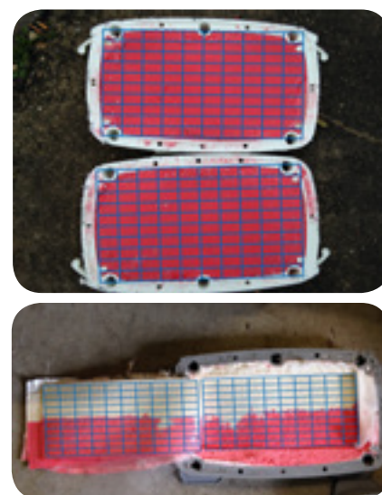
Figure 3: Heatmap of Pod wetting after flushing with current recommended procedure (Left). On the right, flushing Millistak+® X0HC at 600 LMH (up, 100 % wetting) and Millistak+® HC Pro D0SP at 85 LMH (Down, 45 % wetting).
