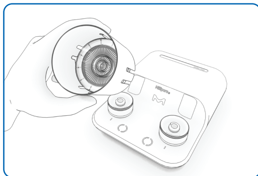
Figure 15b: Membrane support tool with attached membrane support after removal from pump head.
