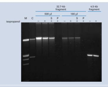
Figure 2: Recovery of DNA fragments extracted from agarose gel slices using the High Pure PCR Product Purification Kit. Samples were processed with isopropanol or without isopropanol. Selected samples were centrifuged at full speed after addition of isopropanol (*S*, supernatant) and the potential precipitates were redissolved in water (*P*, precipitate). As a control (*C*), *Pac* I digested CMV-pAdEasy-1 plasmid DNA was used (*M*, marker: λ *Hind* III-*Eco* RI DNA).
